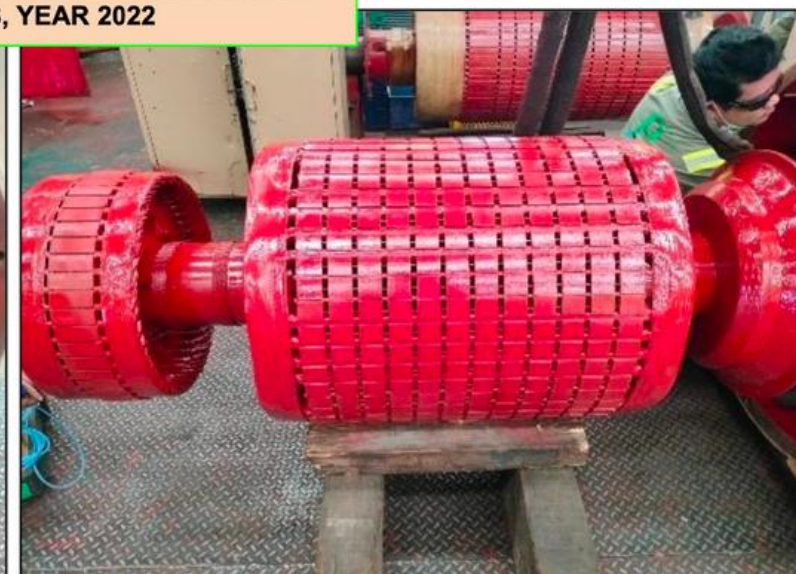
"MITSUBISHI" AC GENERATOR OVERHAULED PROCESS, YEAR 2022
