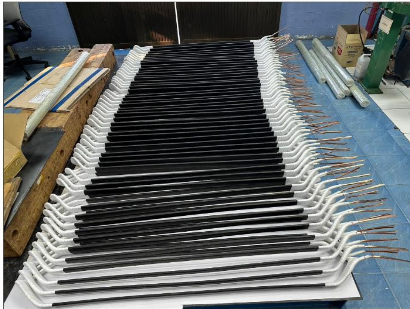
MALAKOFF POWER BERHAD Manufacture coil – Completed coil
