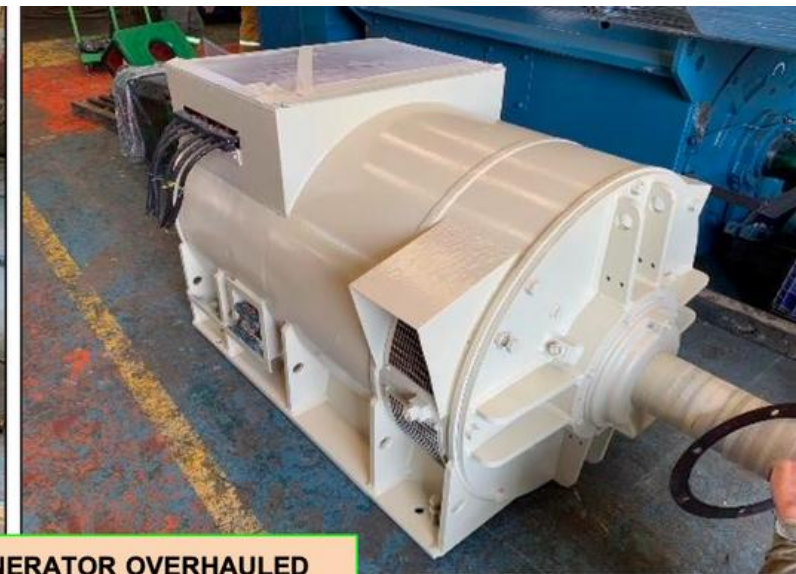
"MITSUBISHI" AC GENERATOR OVERHAULED PROCESS, YEAR 2022
