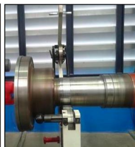
Dynamic balancing main rotor winding with dynamic balance machine "SCHENCK" (Tolerance accord to ISO 1940, Quality grade:G 2.5)
