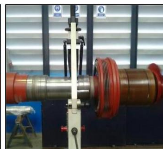
Dynamic balancing main rotor winding with dynamic balance machine "SCHENCK" (Tolerance accord to ISO 1940, Quality grade:G 2.5)
