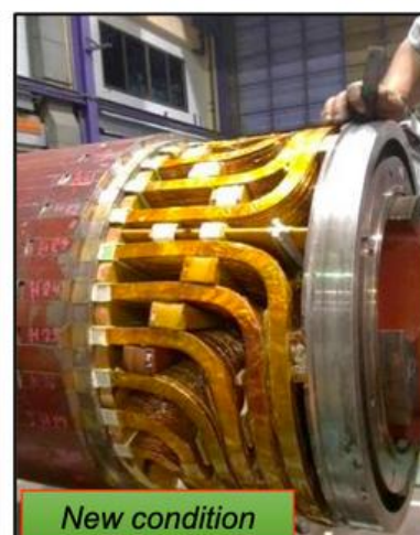
Inserted coil after re-Insulation all new to slot
